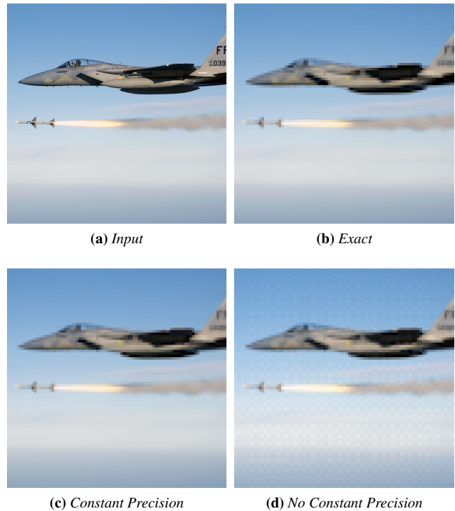
Figure 3: The difference between enforcing constant precision when downsampling an image and not enforcing constant precision with Lanczos 2 filtering.
